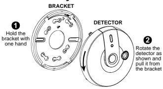
Figure 2. Separating the Detector from Its Bracket
