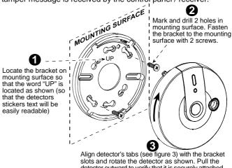
slots and rotate the detector as shown. Pull the detector outward to verify that it is securely attached.
