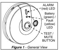
The detector is continuously self-tested and has a TEST button that enables the user to test the detector anytime.
