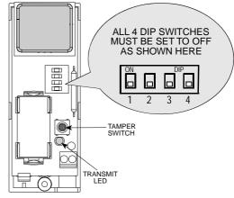
Figure 6. DIP Switches - Correct Position
