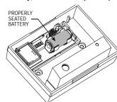
Figure 7. Battery Insertion
