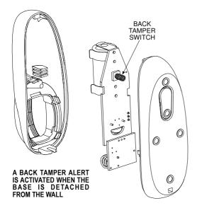
Figure 8. Back Tamper (Rear) View
