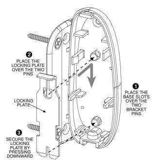
Figure 12. Securing Locking Plate to Base
