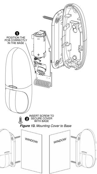
**Note:** The CLIP MCW can be mounted on either side of a window. **Figure 14.** Mounting on Both Sides of a Window
