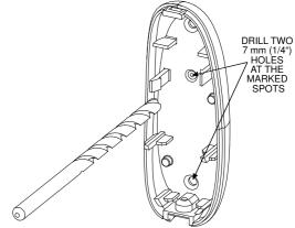
Figure 10. Drilling Holes
