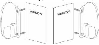
Note: The CLIP MCW can be mounted on either side of a window.
