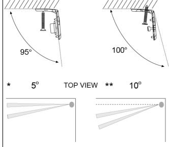
Figure 11. Mounting Bracket to Surface
