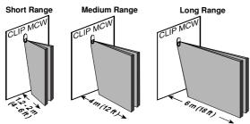
Figure 16. Range Setting Diagram
