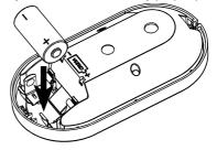
Figure 6 - Battery Insertion
