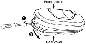
Figure 3 - Rear Cover Removal
