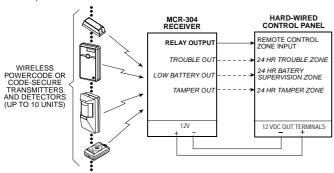
Figure 1. Typical Application of the MCR-304
