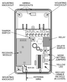
Figure 2. MCR-304 with Cover Removed
