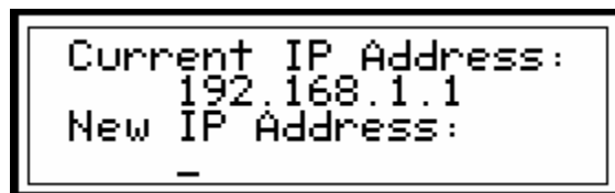
Figure 16- Set IP Address from LCD and keypad
