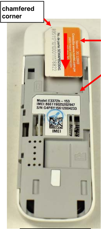
3- Set SIM card on modem above card slot. The chamfered corner is at top left.
