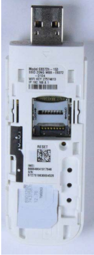
4- Slide SIM card into slot fully. (Card is fully in slot above)
