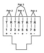
WARNING: The CATx connection cable used between the NTI XTENDEX Series Local Unit and Remote Unit or any XTENDEX Series products must be wired straight through (pin 1 to pin 1, pin 2 to pin 2, etc.) The use of a CROSSOVER CABLE will damage the extender and void your warranty.
