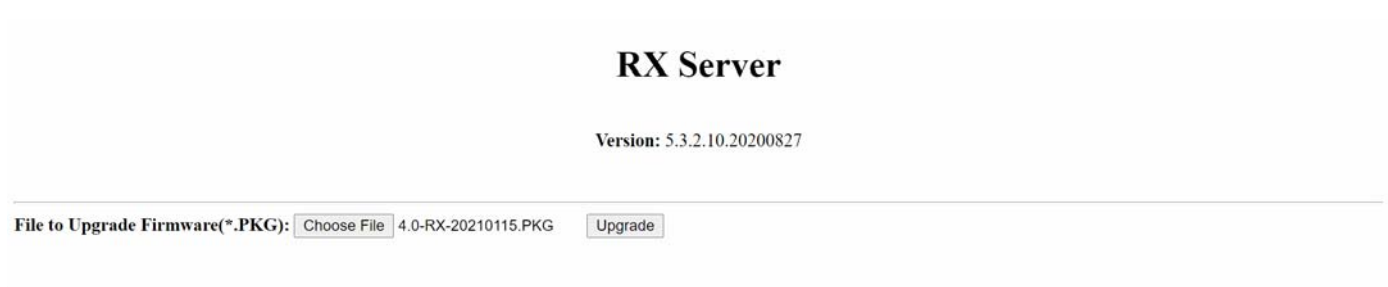
Figure 10- Step one- Open the Upgrade Firmware webpage
