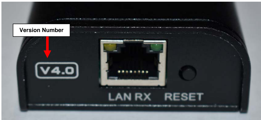
Figure 7- End View of Extender showing version number
