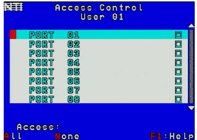
Figure 32- Access Control list
