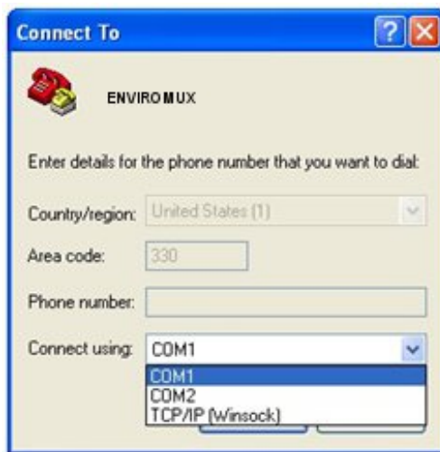
Figure 11- Configure COM port in HyperTerminal
