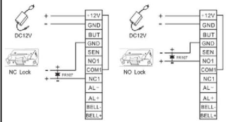
Device share power with the lock: U100K=12V, HLOCK>1A... 1 And the lock is near to the device.
