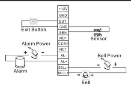
Voltage output ≤ DC 12V for Alarm and Bell
