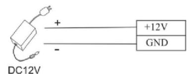
Input DC 12V, 500mA (50mA standby) Positive is connected with **+12V**, negative is connected with **GND** (do not reverse the polarities).
