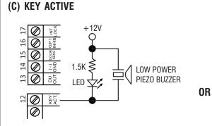
The Key Active Output will switch to (-) ground for 10 seconds whenever a key is touched. You may use it to turn ON an LED lamp and /or a small buzzer to notify a guard; or to energize a relay to switch ON lights or trigger an CCTV Camera to start recording.
