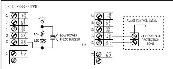
The Duress Output will switch to (–) ground when duress code is entered. You may use it to turn ON an LED lamp and / or small a buzzer to notify a guard; or connect it to a 24 hour Normally Open protection zone of an alarm system.
