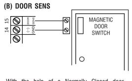
With the help of a Normally Closed door position sensor (usually a magnetic door switch) on the door to set up the following functions:
